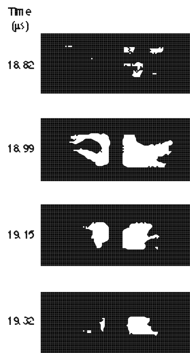
Figure 1. Implosion of a Thin Foil Cylinder at Pegasus II
