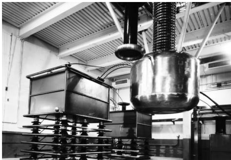
The Illinois Cockcroft-Walton Accelerator. This accelerator was used by John Manley and his group to investigate the efficacy of different metals as a “tamper”—a liner surrounding the nuclear explosive that acts as a neutron reflector and makes the explosive chain reaction more efficient. Gold, uranium, platinum, tungsten, and other metals were investigated as possible tampers.
